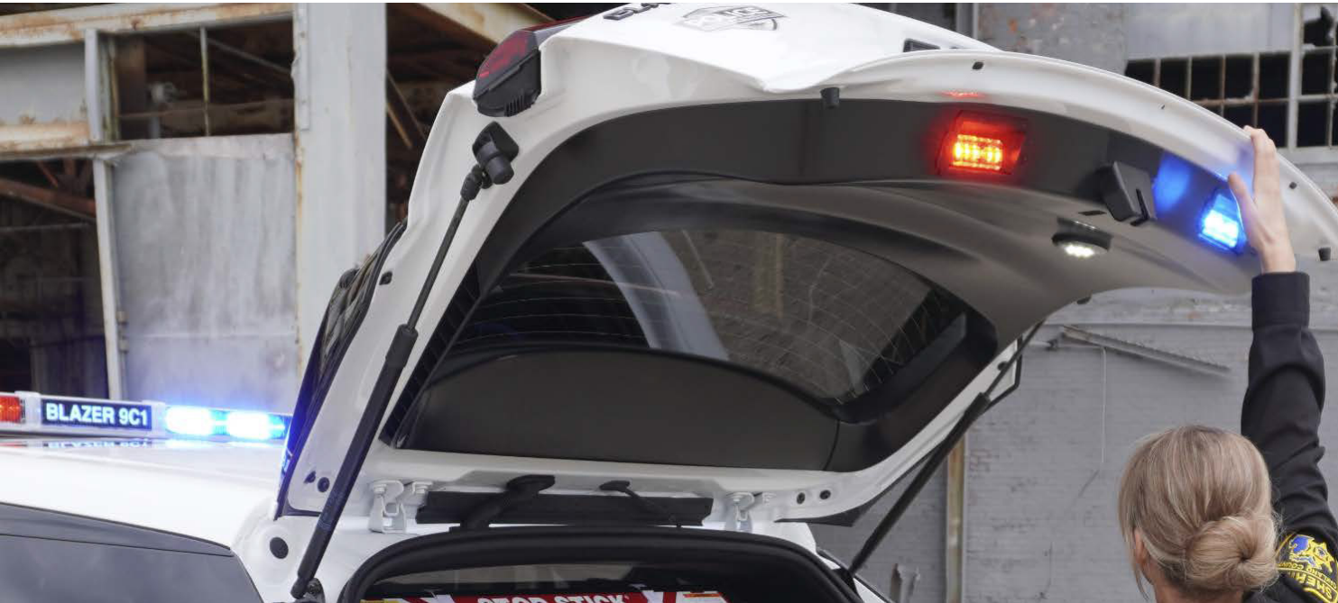
T53 REAR LIFTGATE WARNING LIGHTS
