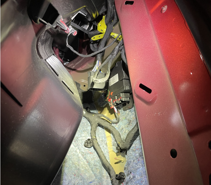
Module and user harness located right rear interior quarter panel.
